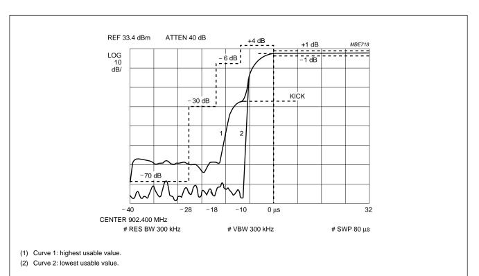
Fig.9 Power as a function of time; rising edge (behaviour at different worst case home positions of V<sub>O(INT)</sub>).
